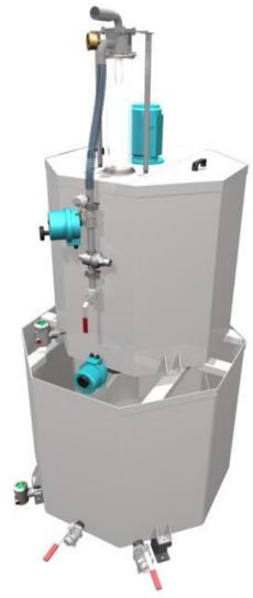
Octopus DT mixes and stores powder polymer solution through a separated two tank system. Powder polymer is transported by air which gives maximum wetting efficiency in the Polywet PPW eductor/wetter. DT is delivered with or without control panel, powder handling, dosing pumps.
